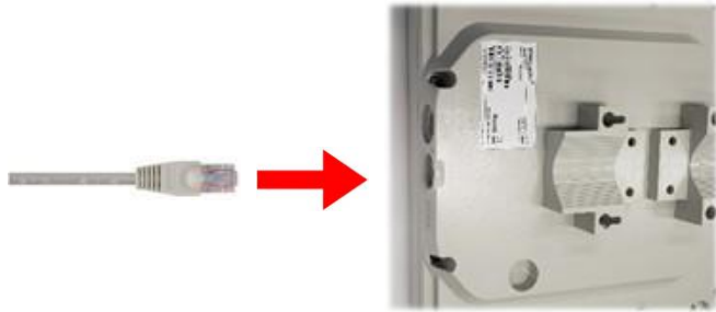
Figure 1 - POE port on bottom of BTI.
