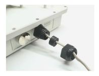
**Step 2:** Push the rubber gasket into the threaded cable guide, then screw the weather shield cap over the threaded cable guide to seal the cable opening.
