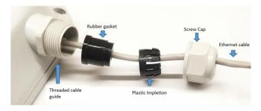
**Step 2:** Push the plastic impletion over the rubber gasket, insert the gasket into the threaded cable guide, then twist the screw cap over the threaded cable guide to seal the cable opening.
